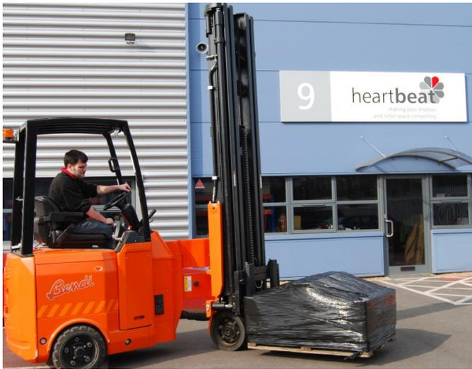
With an aisle width of only 1800mm and a top beam height of 7000mm, the new warehouse is certainly different from the old steel bulk store but the operators had no problems adapting to the new environment or higher lift Bendi's.
